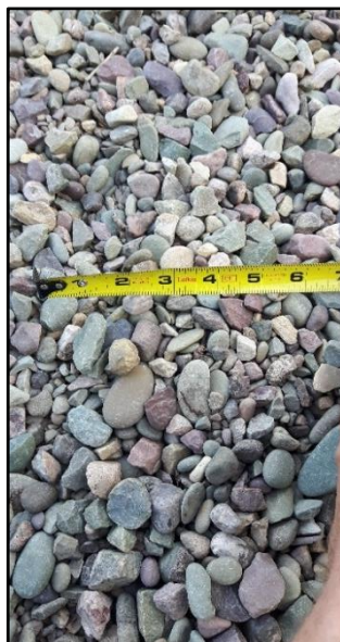
0.5" – 2" gravel/washed rock (inner loop of existing trail)
